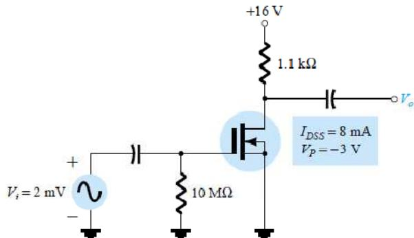
$$r_d = \frac{1}{y_{os}} = \frac{1}{20 \mu\text{S}} = 50 \text{ k}\Omega, V_{GSQ} = 0 \text{ V}$$
