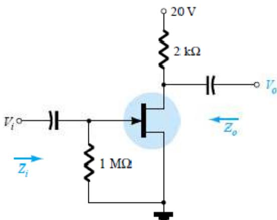
$$V_{GSQ} = 0 \text{ V}, g_m = g_{m0} = \frac{2I_{DSS}}{|V_P|} = \frac{2(6 \text{ mA})}{6 \text{ V}}$$
