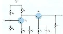
The low voltage gain of the input stage reduces the Miller input capacitance, making this combination suitable for high-frequency applications.
