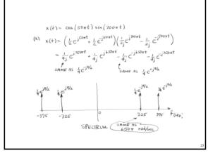
P-4.9 The spectrum diagram gives the frequency content of a signal.
