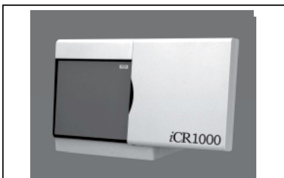
Figure 12.8 Table-top Computed Radiography Cassette Scanner. The screen is removed from the cassette, scanned, erased and returned to the cassette for the next exposure. The image information is sent to a computer for display and analysis. Photo courtesy of iCRCo.
