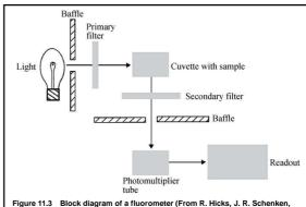
Figure 11.3 Block diagram of a fluorometer (From R. Hicks, J. R. Schenken, and M. A. Steinrauf, *Laboratory Instrumentation*. Hagerstown, MD: Harper & Row, 1974. Used with permission of C. A. McWhorter.)
