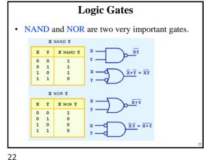
**Logic Gates** • NAND and NOR NOT X are known as x universal gates because they are X AND Y inexpensive to manufacture, and X OR Y any Boolean function can be constructed using only NAND or only NOR gates.
